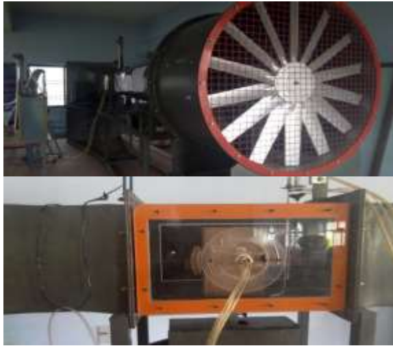
Figure3. Typical views of the instrumented building model inside the wind tunnel.
